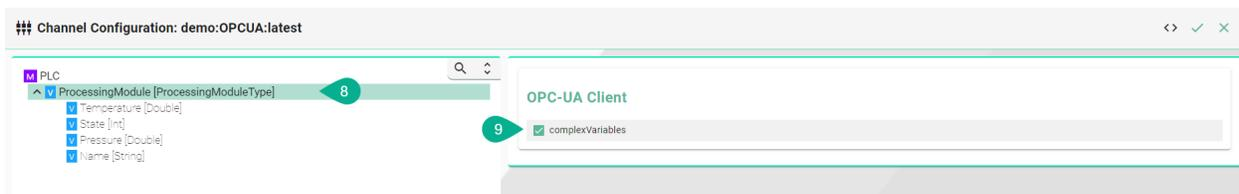
10. Assign OPC-UA data block variables to corresponding variables in the Information Model by selecting the variable in the tree
